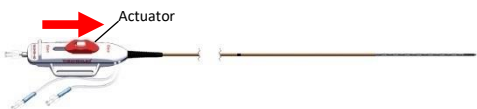
Figure 3. Move actuator in the distal direction while simultaneously pressing the actuator release button to reduce the diameter of the infusion basket. Move actuator fully in the distal direction to completely collapse the infusion basket.
