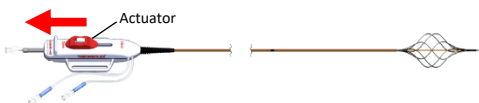
Figure 2. Move actuator in the proximal direction to expand the infusion basket to the desired diameter (diagram not to scale).
